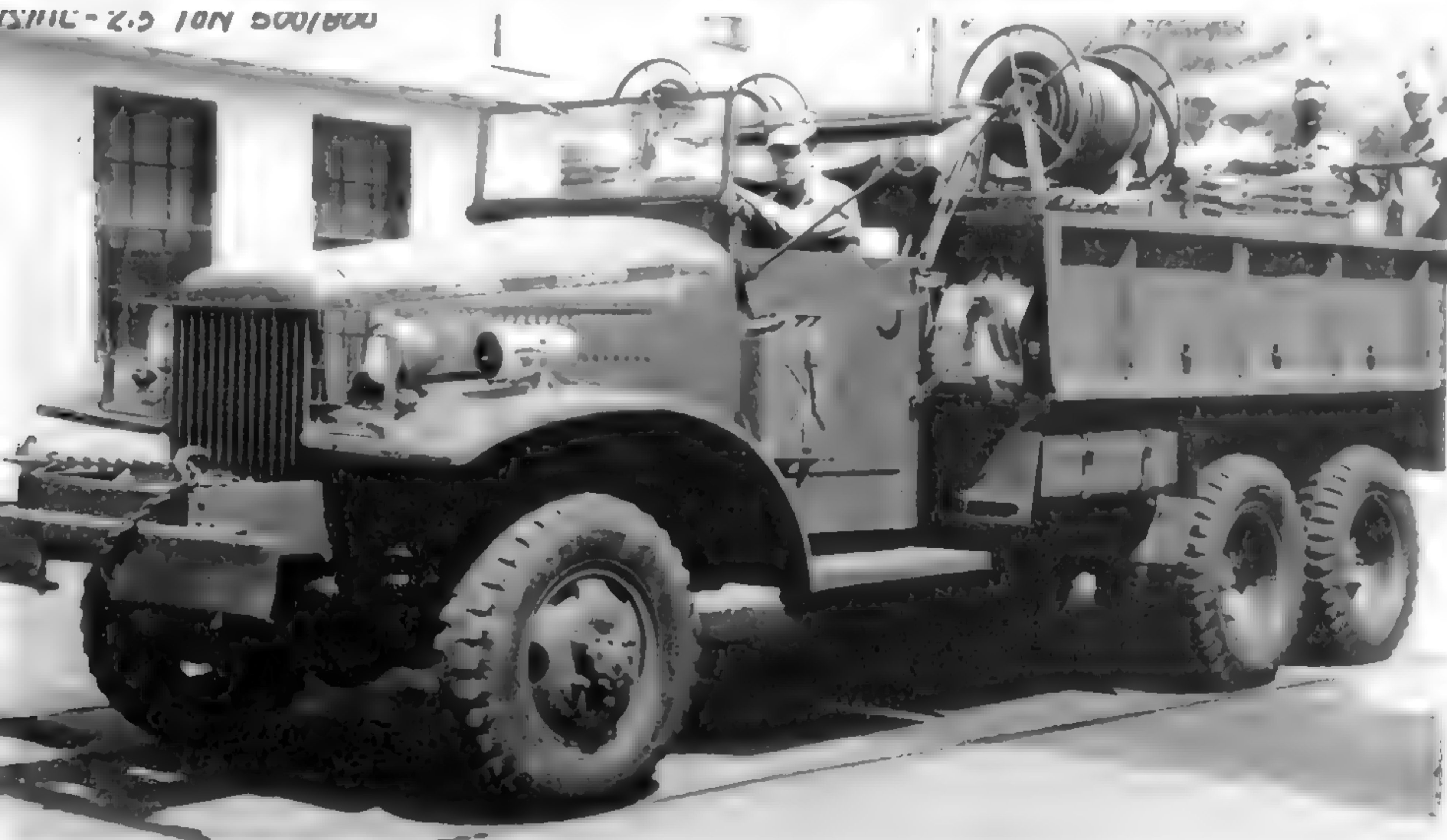
Marines used the International 6x6s for many purposes, including adaptation to fire trucks. (Photo courtesy of Richard Adelman collection)
